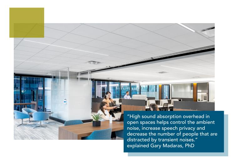
Along with acoustic performance, Rockfon's ceiling systems support sustainability by maximizing the ample Atlanta sunshine radiating through the floor-to-ceiling windows with views overlooking the city. Rockfon Sonar panels' white surface reflects up to 85% of light, extending the daylight more deeply into the office's core. Relying on more natural light reduces the building's electrical and HVAC loads, energy use, and the associated emissions and costs.
